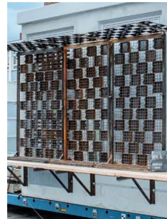
Internal arc fault test arrangement according to IAC-B 20 kA 1s for protection of the public
